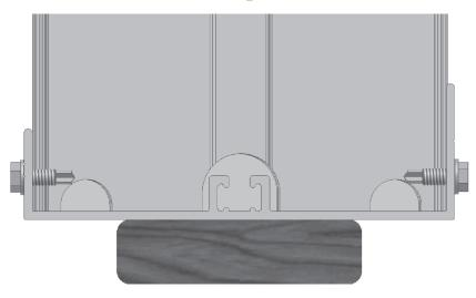
After removing door from carton, move it as close as possible to where it will be installed. Then remove packing support-board under threshold. After it has been removed, move the door as little as possible to put into position.
