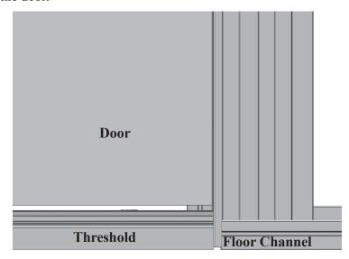
Note: The door panel sub-assembly may be slightly taller than adjacent panels to ensure proper door threshold clearance.
