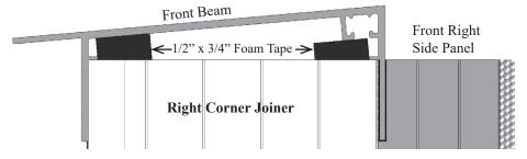
3. Working inside the room, fasten Beam in place with #12 x 3/4" Self-Drilling Screws at corners and at each Panel Frame where they join. It is suggested the screws be installed in the wider leg of the Panel Frame. Screws are installed outside the room and are placed in the same location as inside the room after the roof is installed. If you are adding a Front Header Extension, please refer to Page 14. Gable End Channel
