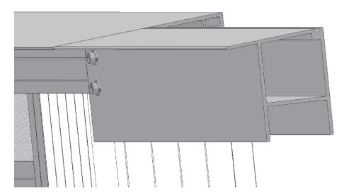
5. Locate and install Post Anchor Bracket on deck or patio. Then locate and install Post(s) using #12 x 3/4" screws to attach to the Roof Header Extension. (See your Roof Installation instructions for Anchor Bracket installation)
