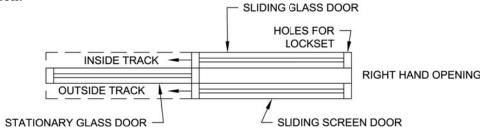
After you have determined whether the Sliding Door is going to open from the Left or Right. Install the Stationary Door in the center track first by inserting the top of the Door into the Door Frame Top Track. If the Sliding Door is right hand opening, slide the Stationary Door all of the way to the left.
