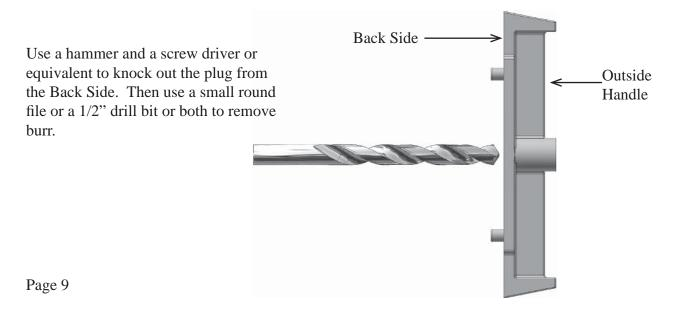
After you knock out the plug, you must clean out the unavoidable burr with a round file or a 1/2" drill bit. Again, be sure to insert the file or drill bit from the **back side** and work it around several times to remove the burr. If the key lock is still difficult to install, make a few more passes with the file or drill bit.
