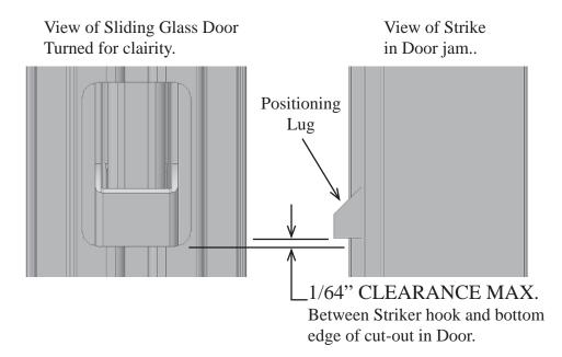
After the Strike has been properly adjusted and tightened, drill a 3/32" hole for the third screw (at top of strike). This screw secures the strike for maximum forced entry protection.
