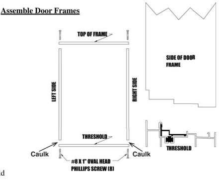
**Note:** High side of threshold is placed inside the room, the same way you installed the Floor Channel.
