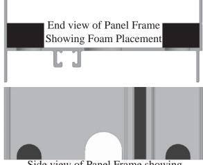
Side view of Panel Frame showing routed holes on Bottom
