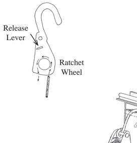
5. Secure hook to Post top as shown in drawing.
