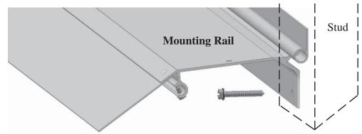
6. Secure the Mounting Rail to the side of the RV with  $#12 \ge 1-1/2$ " screws. Mark the locations of all studs or solid support on the bottom lip of the Mounting Rail. Drill 7/32" holes through your marks on the Mounting Rail. Install  $#12 \ge 1-1/2$ " screws. If you must shim the Mounting Rail, you should replace the  $#12 \ge 1-1/2$ " screws provided with new screws of an appropriately longer length.
