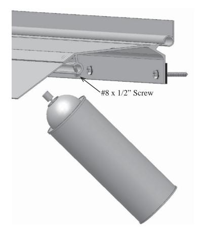
**2**. Remove the factory installed #8 x 1/2" Screw Stop at the Right End of the Mounting Rail. This will allow you to insert panels. Save the #8 x 1/2" Screw Stop because you will replace it after all awning panels have been installed.
