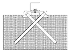
**2**. Drive two (2) Soil Anchor Pins alternately until flush with Anchor Base.
