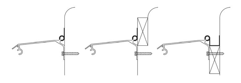
**3**. Because there are various styles of awning rails it may be necessary to shim either the RV Rail or the Dura-Fold Mounting Rail. See drawings above. Shim material is not provided with the Awning. **Caution!** Make sure when you are completed with this step that the Dura-Fold Mounting Rail is below horizontal or water will run back to RV wall and cause leaking.
