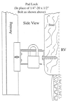
**3**. Fasten the 1-1/2" x 2-1/2" Angle to the Lock Down Clip with 1/4"-20 x 1/2" Hex Head Bolt and Wing Nut. Make sure to attach Angle so the 1-1/2" leg faces down.
