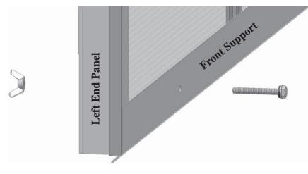
**5**. Install 1/4-20 x 2" Aluminum Hex Head Bolt, EPDM Washer and Wing Nut in each hole, making sure the Wing Nut is on the underside of the awning.
