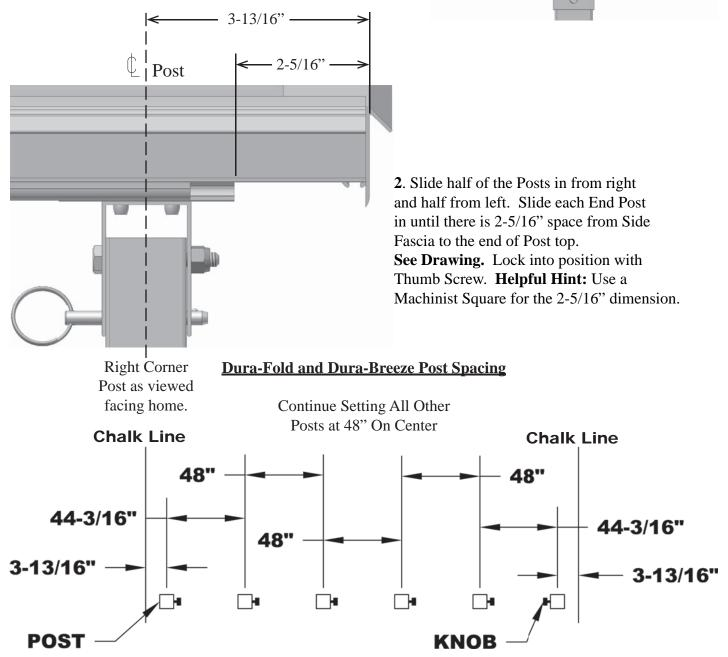
**Helpful Hint:** As you slide Posts into the Track be aware of the position of the Knob on the Post. The Corner Posts need the Knob to be facing away from the corner. To accomplish this you must disassemble the post top and rotate it 180°. (See Drawing Above)
