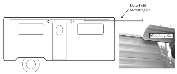
**4**. Slide the Left End Dura-Fold Mounting Rail section into the RV awning rail until it reaches the thumb screw stop you installed.
