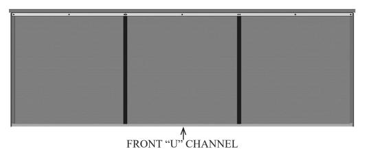
7. Install the Front Trim over the "U" Channel and fasten the Front Trim, Left and Right Trims using #8 x 1/2" screws. As shown below. (Make sure the screws go thru the Trim, "U" Channel and Slide Out Roof Panel)
