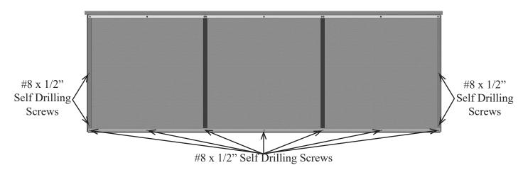
**8.** Use #8 x 1/2" screws to fasten the Front Trim, Left and Right Trims underneath. Install two (2) one in each corner going up through the bottom of the Mounting Rail. See Below.
