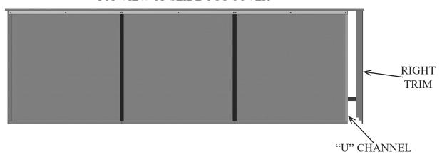
**6.** Install "U" Channel over the front of all Slide Out Roof Panels. (Do not use any fasteners at this time) TOP VIEW OF SLIDE OUT COVER
