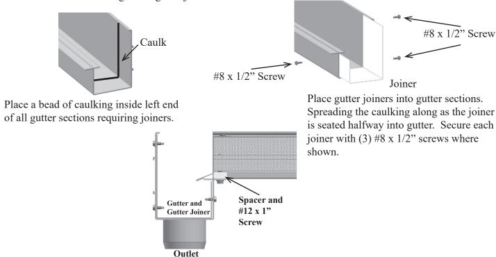
Attach Right Gutter Section to Right Side Fascia and Girder, including a Hard Plastic Spacer, with a #12 x 1" Self Drilling Screw. **See Drawing.**
