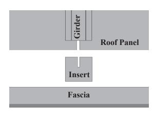
As with the Side Fascias, apply a bead of caulk on the top of each roof panel about 1/2" in from edge. Then slide Fascia onto the Panel ends.
