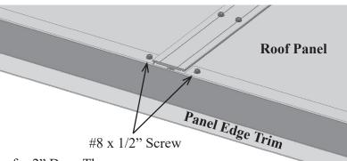
Panel Edge Trim is supplied in 120-15/16" lengths for 2" Dura-Therm and 109-3/16" lengths for 3" Dura-Therm. Cut last section to fit Roof length.
