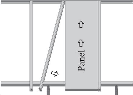
Move the free end of the second Girder to your lett. This will form a "V" shaped opening. See illustration. Insert Roof Panel into edges of the first and second Girder as close to Mounting Rail as possible. As Roof Panel is pushed into Mounting Rail, pull the free end of the Girder against and on the Roof Panel. Guide Girder on Panel, being careful not to damage the skin of the Panel.
