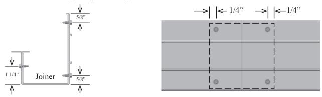
When gutter is aligned and bolted to each girder with 1/4"-20 x 1/2" hex head bolt and nut, fasten joiner(s) into place with #8 x 1/2" screws as shown.
