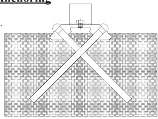
Note: The Soil Anchor Pins are 1/2" dia. x 24" long Oval Head Round Steel Pins made from C-1018 Material entering the soil @ 45°.
