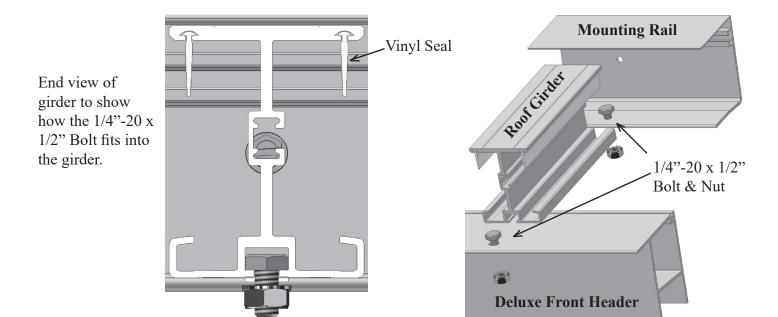
Insert bolts in every hole in Mounting Rail. Lay first Girder on the Front Header and pull it back into the Mounting Rail. Do not position a Girder at the ends of the roof, they will be finished with Side Fascias after all Girders are installed. Hold bolt in Mounting Rail up enough to guide bolt head into "T" slot of the Girder. Push Girder fully into Mounting Rail. Hand tighten nut.
