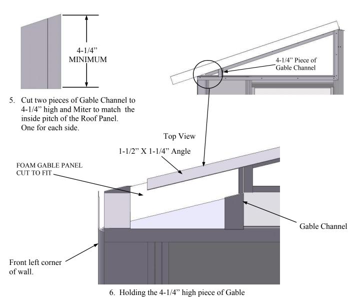
Channel in place you must now measure the small area in the corner for a piece of Gable Panel to be cut to fit in this area on both sides.
