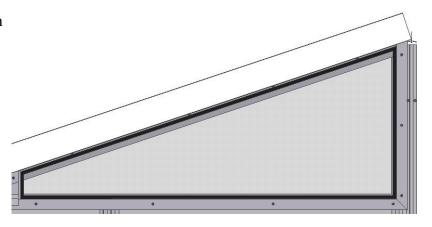
13. Use the 1-1/2" X 1-1/4" Angle and Apply a fine bead of caulk to the 1-1/4" surface of the angle that will be against the roof panel and in the corner where the glass meets the roof. Use #8 X 1/2" screws to attach the angle in place.
