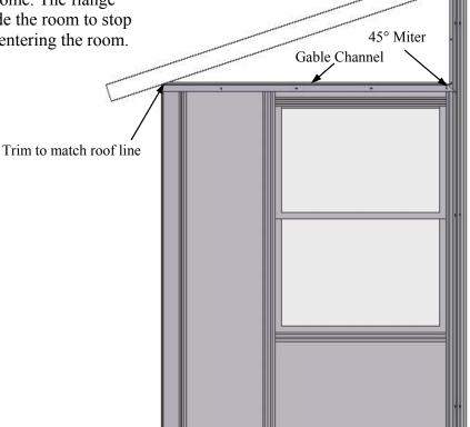
2. Install the Gable Channel that will be attached with #8 X 1/2" screws vertically on the left and right side of the Center Support Column. These pieces will also have to be mitered
