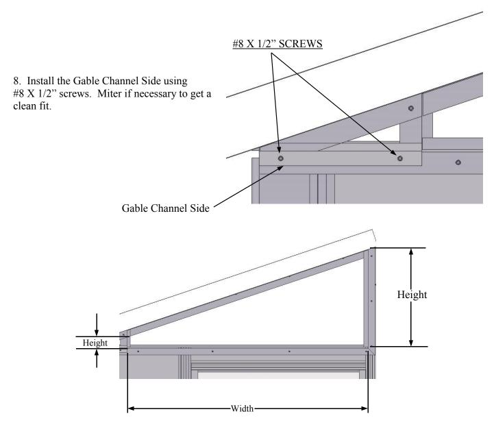
9. To make the Cardboard Template that must go to the glass supplier. Measure the opening for both sides, Width and Height and Subtract 1/4" from the width and the height.
