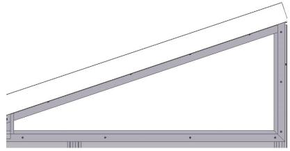
12. Slide the Glass into the opening. from the outside. The rest of the enclosing Angle will be installed from the outside.
