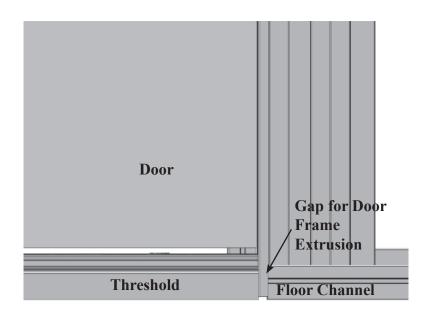
Note: The aluminum nose of the threshold always faces to the outside. If the Door is in-swinging the threshold will have to be notched to allow the adjustable rail to be under the door.
