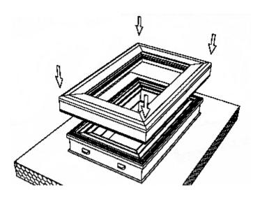
Fasten sash to main frame in pre-drilled holes located on hinge using fasteners supplied.
