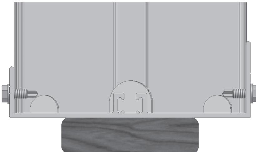
After removing door from carton, move it as close as possible to where it will be installed. Then remove packing support-board under threshold. After it has been removed, move the door as little as possible to put into position.
