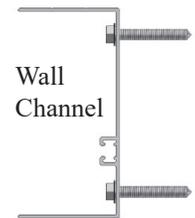
(without the Panel Frame) into the Wall Channel. The Bottom of Panel Frame has holes cut to fit thermal barrier and screw heads in Floor Channel. (See Illustration 1) Seat the Panel in the Floor Channel. Do not fasten Starter Panel in Wall Channel at this time. Insert Panel Frame Insulator into the Panel Frame on the Starter Panel.
