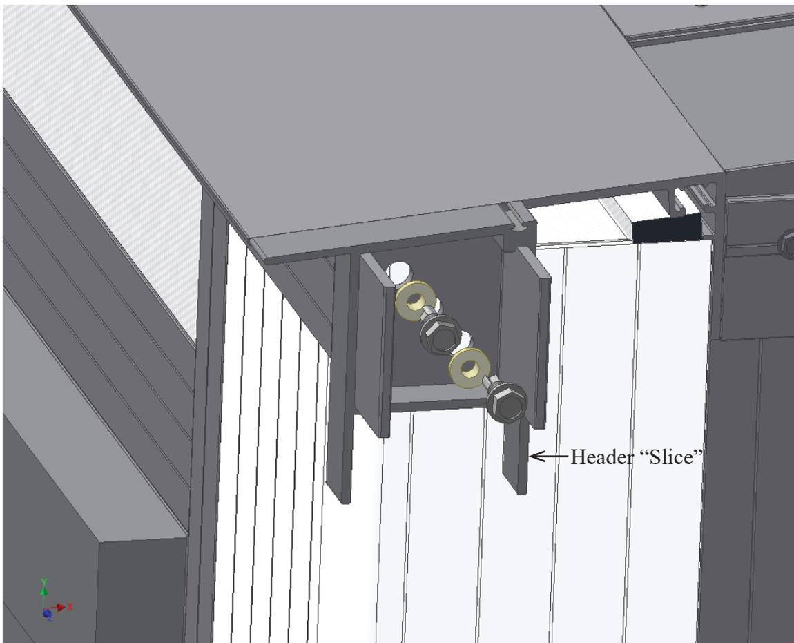
4. Remove Header “**Slice**” (it is no longer needed) and install the Header. Secure the Header to the Joiner with four (4) #12 x 3/4” Self Drilling Screws . . .two (2) in the front side and two (2) in the back side of the Header.
