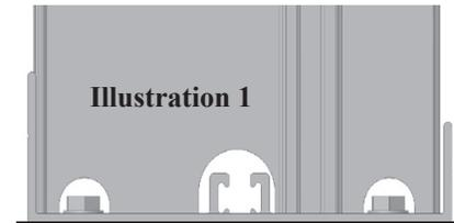
**Helpful Hint:** Use your fingers to break out a piece of foam, (3/8" x 5/8") to give thermal barrier clearance in Floor Channel. Tape Panel Frame Insulator in position while installing next panel.
