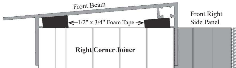
3. Working inside the room, fasten Beam in place with #12 x 3/4” Self-Drilling Screws at corners and at each Panel Frame where they join. It is suggested the screws be installed in the wider leg of the Panel Frame. Screws are installed outside the room and are placed in the same location as inside the room **after the roof is installed.** If you are adding a Front Header Extension, please refer to Page 14. Gable End Channel
