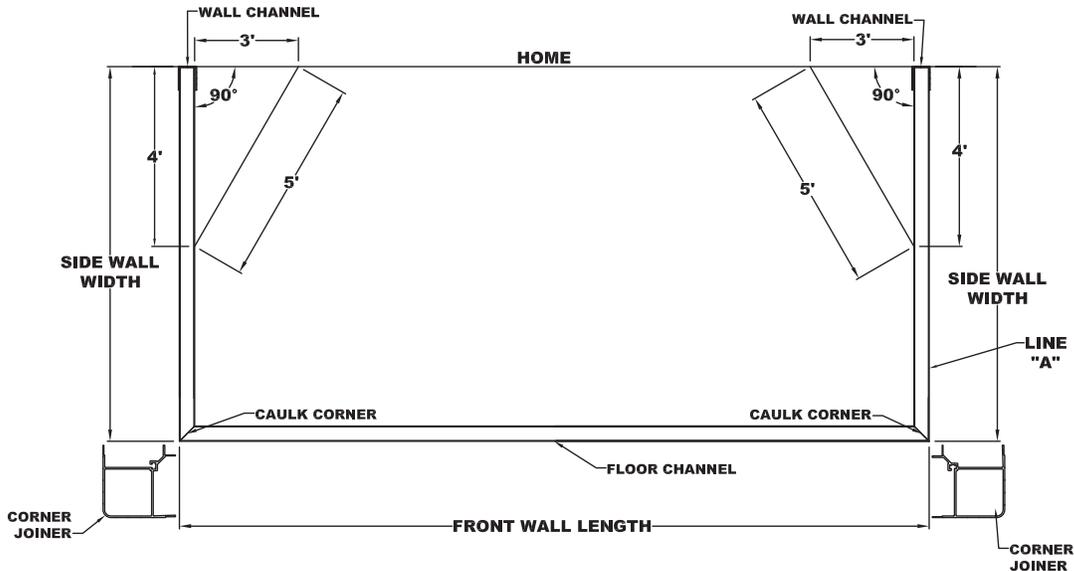
2. Determine the location of the back Left Corner of the room. (Use the Front Wall Length given in your Project Planner as a guide.) Mark the Left Side Wall with a chalk line the same way you marked the Right Side Wall.
