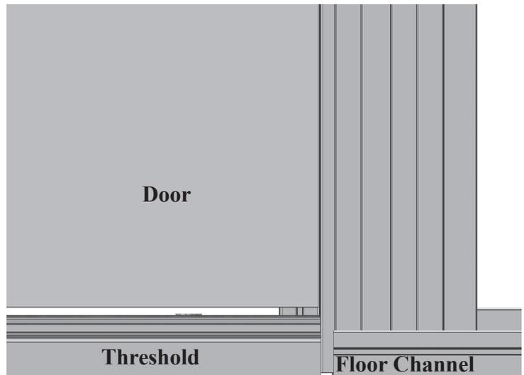
Note: The door panel sub-assembly may be slightly taller than adjacent panels to ensure proper door threshold clearance.
