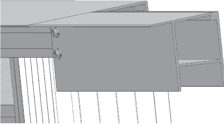
5. Locate and install Post Anchor Bracket on deck or patio. Then locate and install Post(s) using #12 x 3/4” screws to attach to the Roof Header Extension. (See your **Roof Installation instructions for Anchor Bracket installation**)
