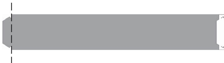
**If you are installing a fan beam, please note that the proper position is to have the beam cavity closer to the top of the panel rather than the bottom of the panel.**
