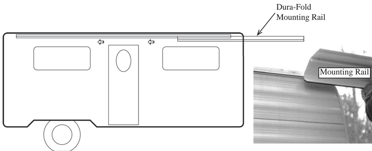
4. Slide the Left End Dura-Fold Mounting Rail section into the RV awning rail until it reaches the thumb screw stop you installed.
