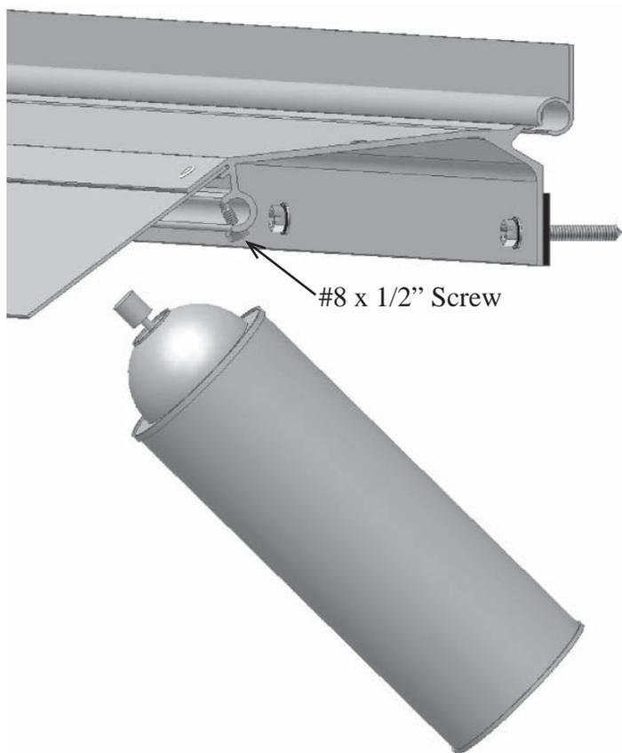
2. Remove the factory installed #8 x 1/2" Screw Stop at the Right End of the Mounting Rail. This will allow you to insert panels. Save the #8 x 1/2" Screw Stop because you will replace it after all awning panels have been installed.
