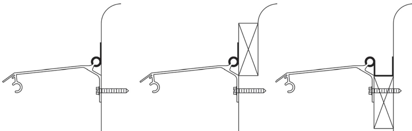
3. Because there are various styles of awning rails it may be necessary to shim either the RV Rail or the Dura-Fold Mounting Rail. See drawings above. Shim material is not provided with the Awning. **Caution!** Make sure when you are completed with this step that the Dura-Fold Mounting Rail is below horizontal or water will run back to RV wall and cause leaking.
