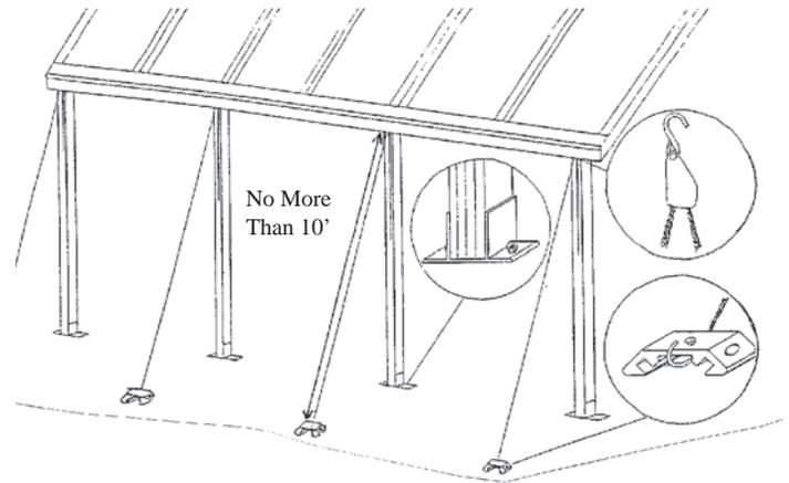
2. Drive two (2) Soil Anchor Pins alternately until flush with Anchor Base.
