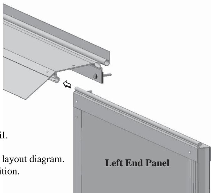
**Helpful Hint:** Panels will tend to slide easier if you keep your hand as high as possible on the edge of the panel while you are pushing it along Mounting Rail. If a panel gets stuck, don't hammer on the panel. Use a rod or rail reamer to drive the bead on the panel along Mounting Rail.
