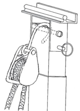
6. Secure other hook to Anchor as shown in drawing. Make sure hook is secured from under side of Anchor. This keeps it from coming loose when tension is applied.
