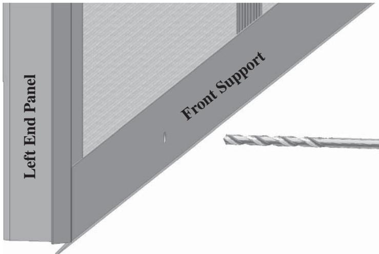
4. Using the pre-drilled holes in the Front Support as a template, drill a 1/4" hole through the panel.
