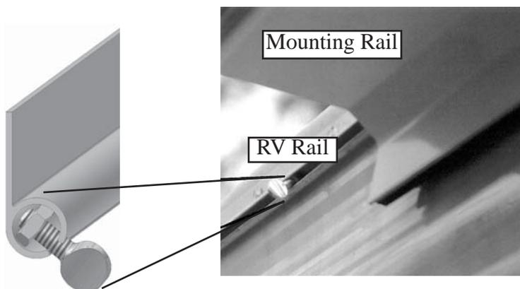
Install 1/2" thumb screw and nut into RV rail. Slide thumb screw to the left end position, mark and tighten. This will stop the Mounting Rail at the proper location.
