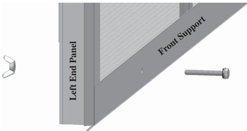
5. Install 1/4-20 x 2" Aluminum Hex Head Bolt, EPDM Washer and Wing Nut in each hole, making sure the Wing Nut is on the underside of the awning.
