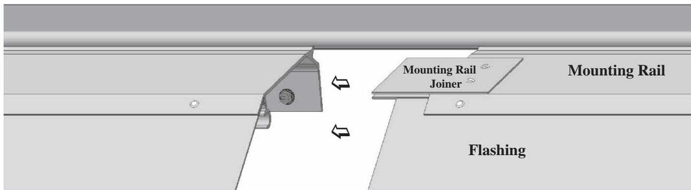
7. If you loosened any fasteners in the RV Awning Rail, tighten them now. First, apply a generous bead of caulking in the cavity between the RV Awning Rail and the side wall of the RV. Also caulk full length of top of the joint of Dura-Fold Mounting Rail and the RV Mounting Rail.
