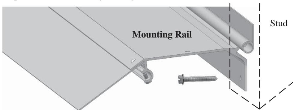
6. Secure the Mounting Rail to the side of the RV with #12 x 1-1/2" screws. Mark the locations of all studs or solid support on the bottom lip of the Mounting Rail. Drill 7/32" holes through your marks on the Mounting Rail. Install #12 x 1-1/2" screws. **If you must shim the Mounting Rail, you should replace the #12 x 1-1/2" screws provided with new screws of an appropriately longer length.**
