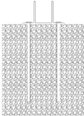
Soil Anchor can **not** be used without Tie Down Kit.
