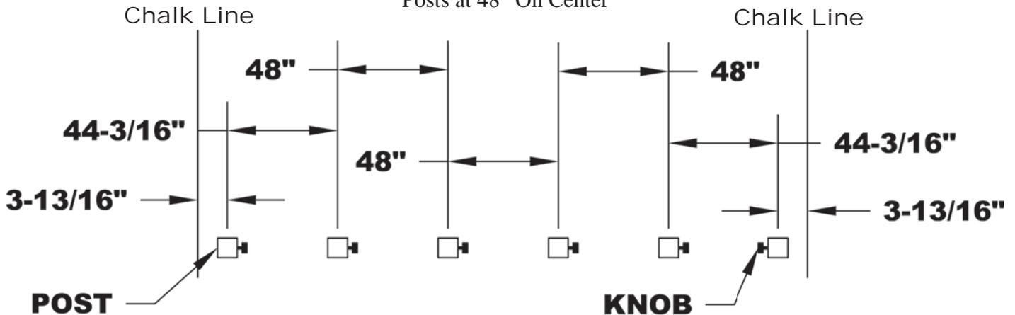
**Helpful Hint:** As you slide Posts into the Track be aware of the position of the Knob on the Post. The Corner Posts need the Knob to be facing away from the corner. To accomplish this you must disassemble the post top and rotate it 180°. (See Drawing Above)
