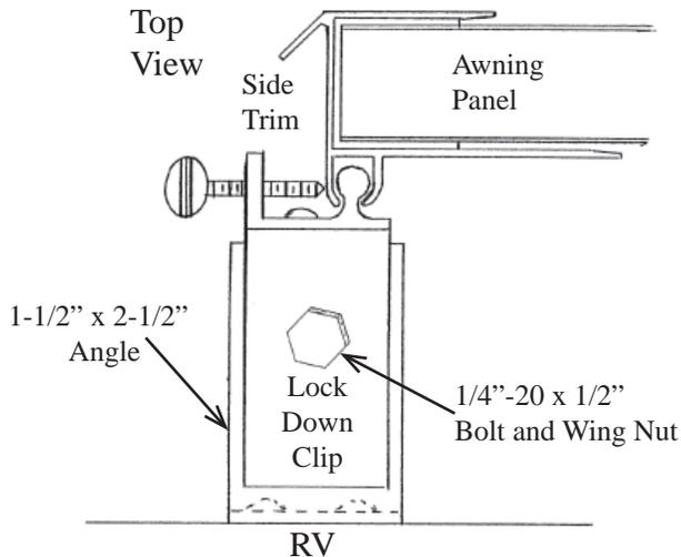
3. Fasten the 1-1/2" x 2-1/2" Angle to the Lock Down Clip with 1/4"-20 x 1/2" Hex Head Bolt and Wing Nut. Make sure to attach Angle so the 1-1/2" leg faces down.
