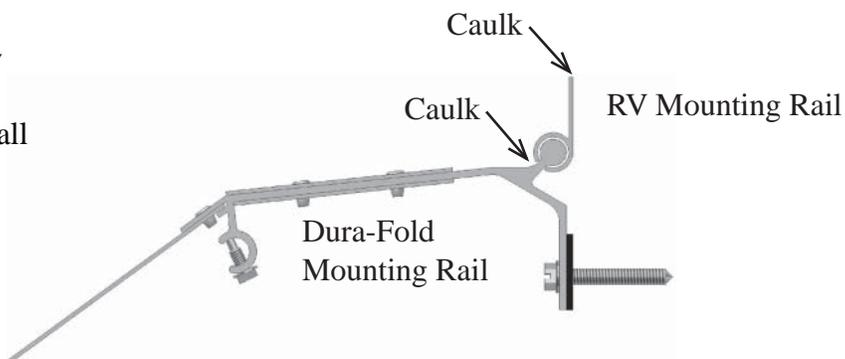
8. After all sections of the Dura-Fold Mounting Rail are installed and the RV Awning Rail has been secured as described in Step 7, apply Sealer Tape. Remove film covering the black, sticky surface. Apply over the center of each joint; covering flashing, Mounting Rail, Mounting Rail Joiner and continuing over the bead of RV Awning Rail. Make sure that tape adheres to all surfaces.
