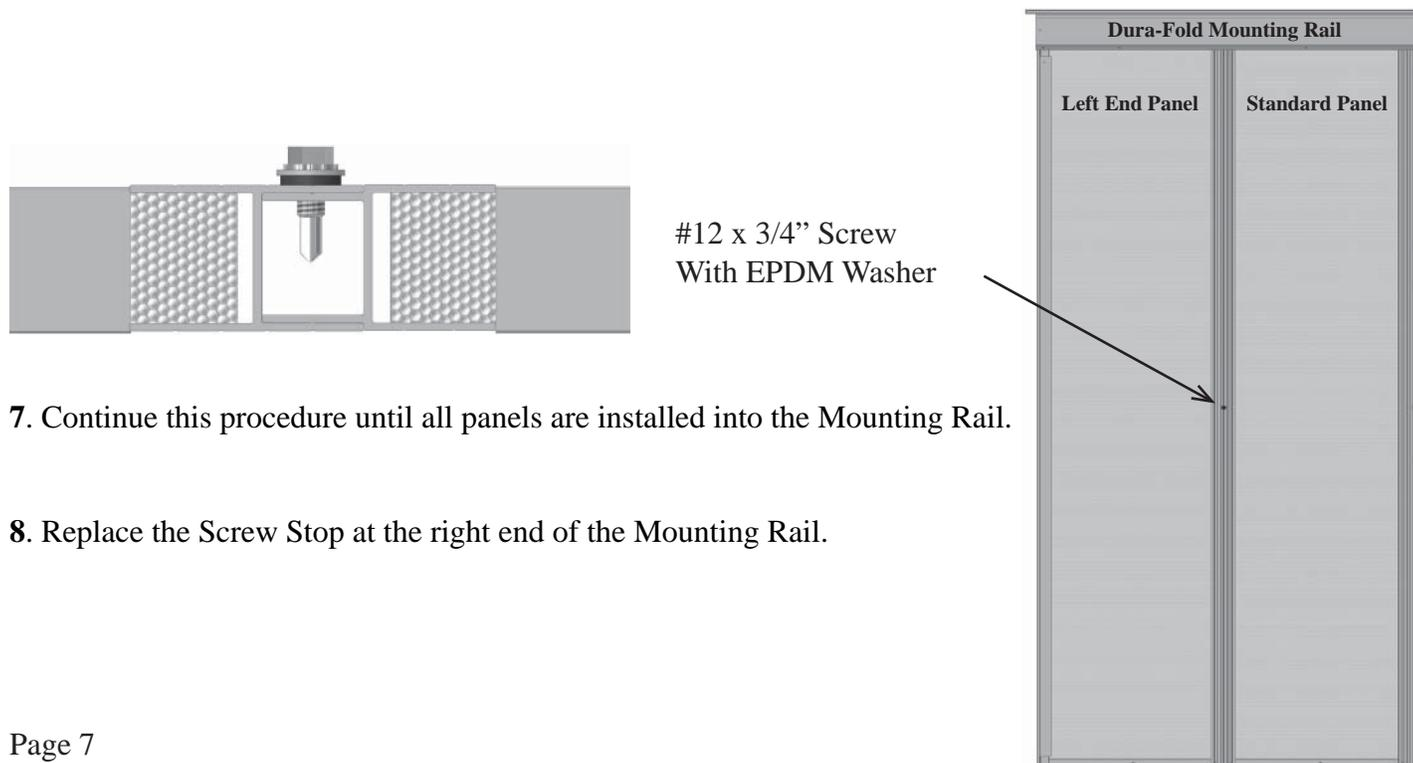
7. Continue this procedure until all panels are installed into the Mounting Rail.
