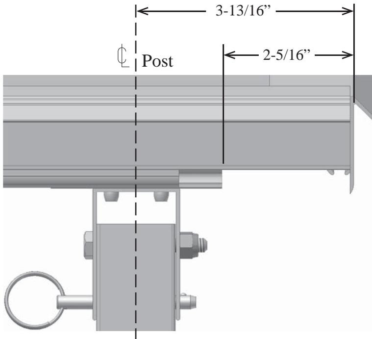
2. Slide half of the Posts in from right and half from left. Slide each End Post in until there is 2-5/16” space from Side Fascia to the end of Post top.
