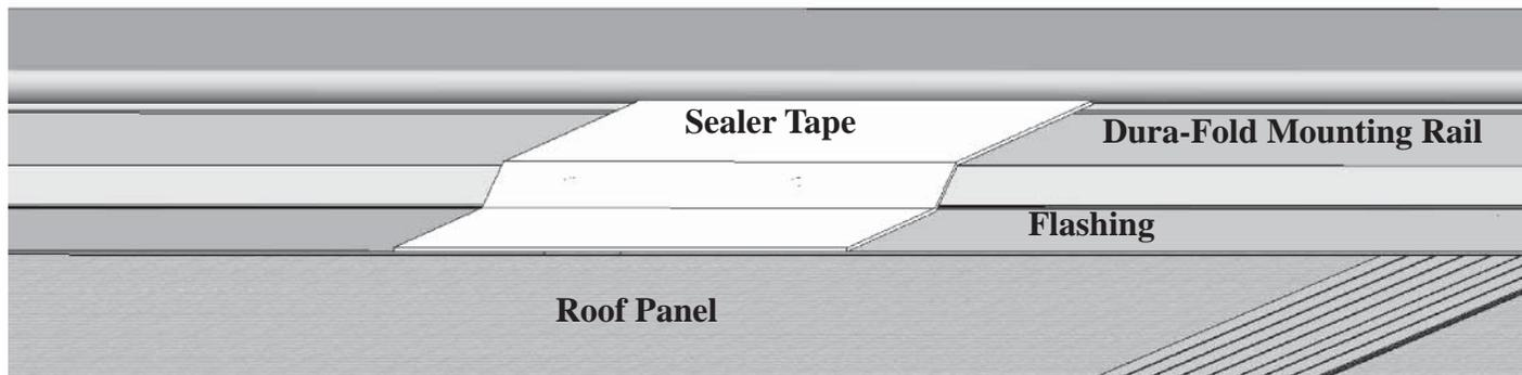
When Dura-Fold Mounting Rail is properly installed as described, the **Mounting Rail** will not need to be removed while transporting the RV over the road.
