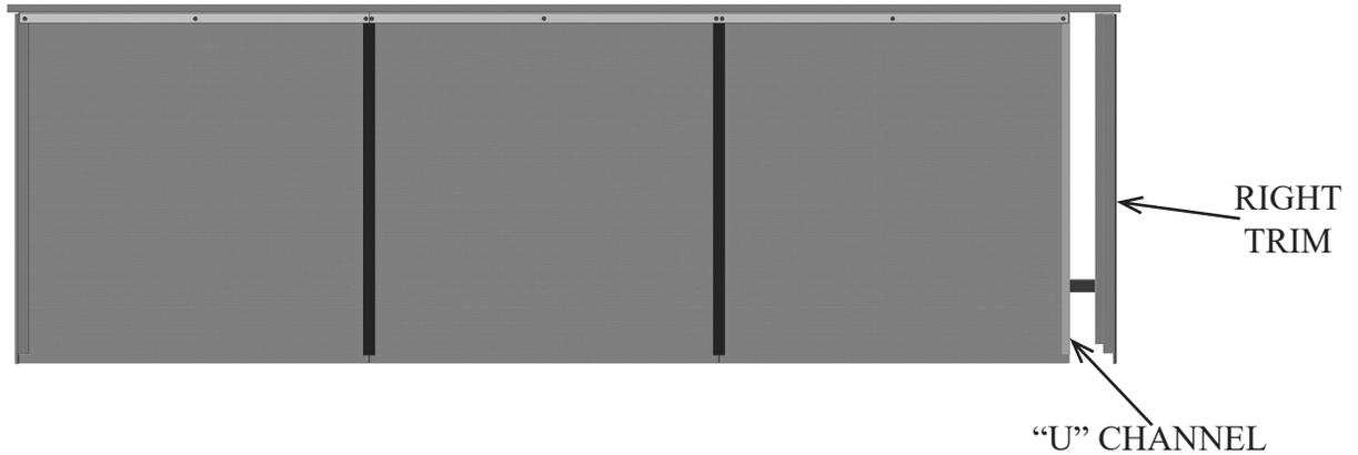
6. Install "U" Channel over the front of all Slide Out Roof Panels. (Do not use any fasteners at this time)
