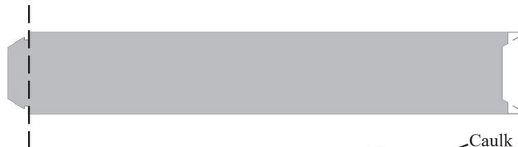
13. Apply a bead of caulk to full length where the top of the Roof Panels meet the Mounting Rail.
