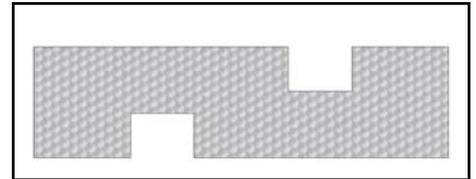
Foam insulation to be installed in the Window Surround.
