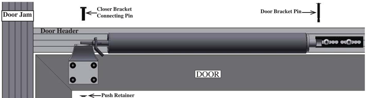
1. Locate and pre-drill the four (4) factory marked Positions with a 9/64" drill. Attach the Closer Bracket to the Door oriented as shown with four (4) Closer Bracket Screws.
