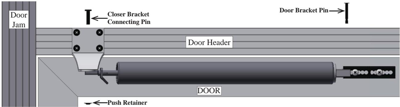
1. Locate and pre-drill the four (4) factory marked Positions with a 9/64" drill. Attach the Closers Bracket to the Door Header oriented as shown with four (4) Closers Bracket Screws.
