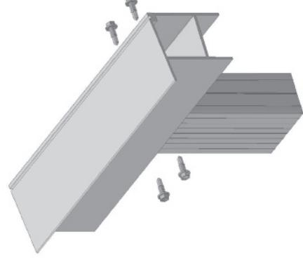
There are two ways to set up your Pillar Columns in relation to the Front Header. See Drawings.
