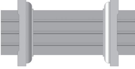
**Note:** If you are installing Pillar Columns on a Pressure Treated Lumber Deck. With your order you will receive a 4" x 4-1/2" piece of Black Flashing with paper coated adhesive on one side for each Pillar Column. Peel the paper off from the Flashing and stick the flashing to the bottom of the Column Angle Brackets. Then trim the excess Flashing from around the Column Angle Brackets.
