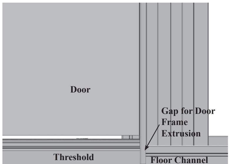
**Note: The aluminum nose of the threshold always faces to the outside. If the Door is in-swinging the threshold will have to be notched to allow the adjustable rail to be under the door.**
