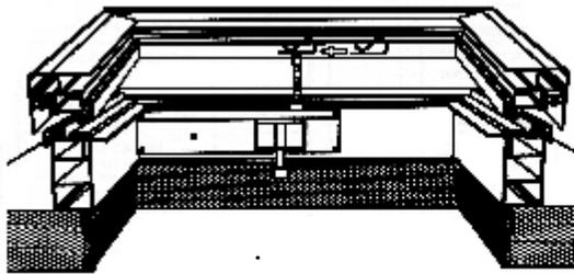
Position the hardware chain link in keeper and insert pin in place
