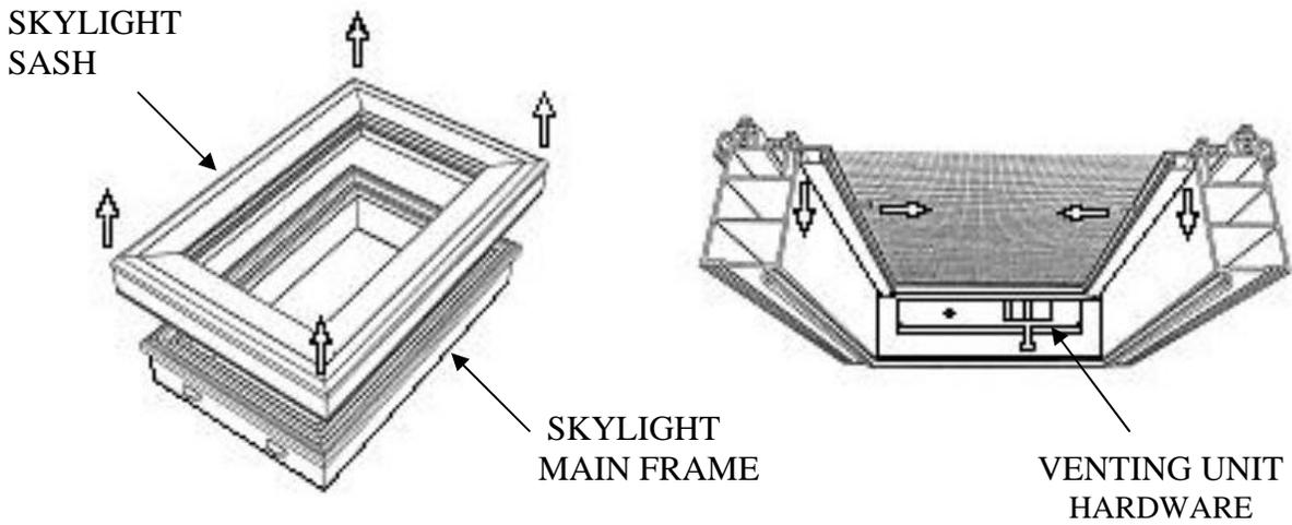
**Handle With Caution!** Venting unit sash is not fastened to main frame on header. Open the venting sash to maximum height, remove pin from hardware, separate sash from main frame and remove insect screen.
