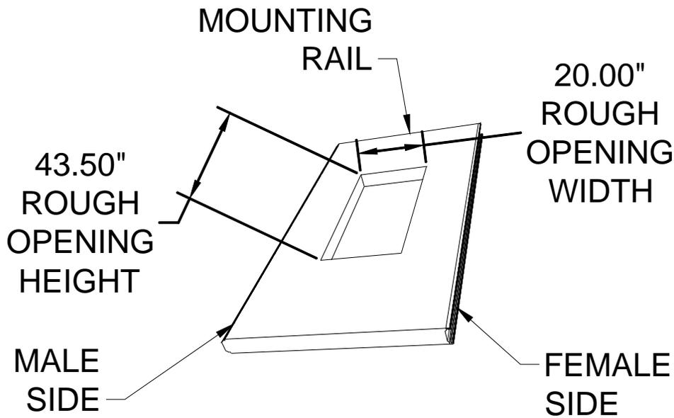
The above illustration shows the standard installation of a Dura-Lock Roof.
