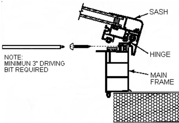
Fasten sash to main frame in pre-drilled holes located on hinge using fasteners supplied.
