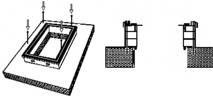
Fasten skylight to roof panel with 3/16" socket drive head. #10 x 5-1/4" screws.
