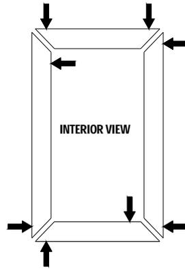
Adjust mitered ends of snap-on covers if required for proper alignment.
