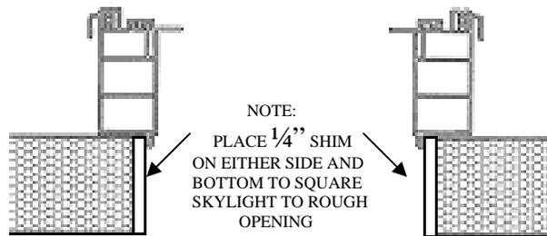
Using 1/4" spacers on either side and bottom, align and square skylight to opening.
