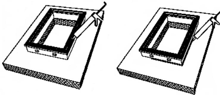
Fill screw holes with white caulk to avoid moisture accumulation.
