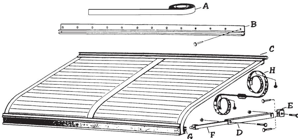
1. Place Weather Strip "A" on back of Mounting Rail "B" if not already installed. Remove protective paper.
