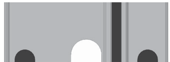
Side view of Panel Frame showing routed holes on Bottom
