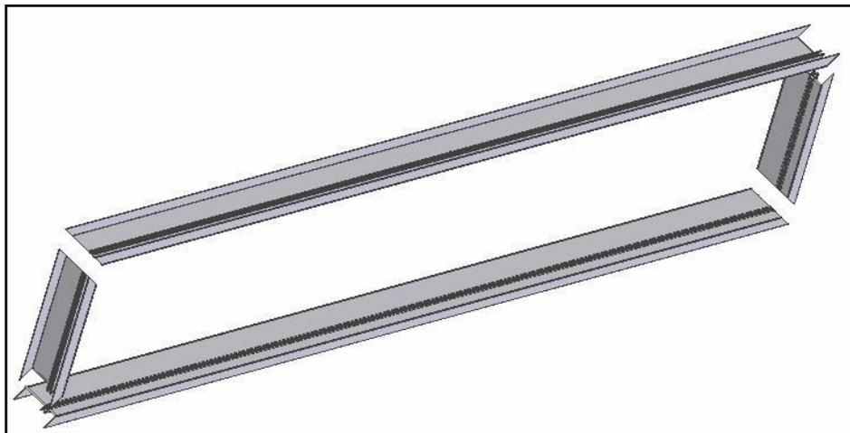
3 ) Install the side pieces of the Window Surround the same as in Step (2) making sure the Thermal Barrier is toward the outside.
