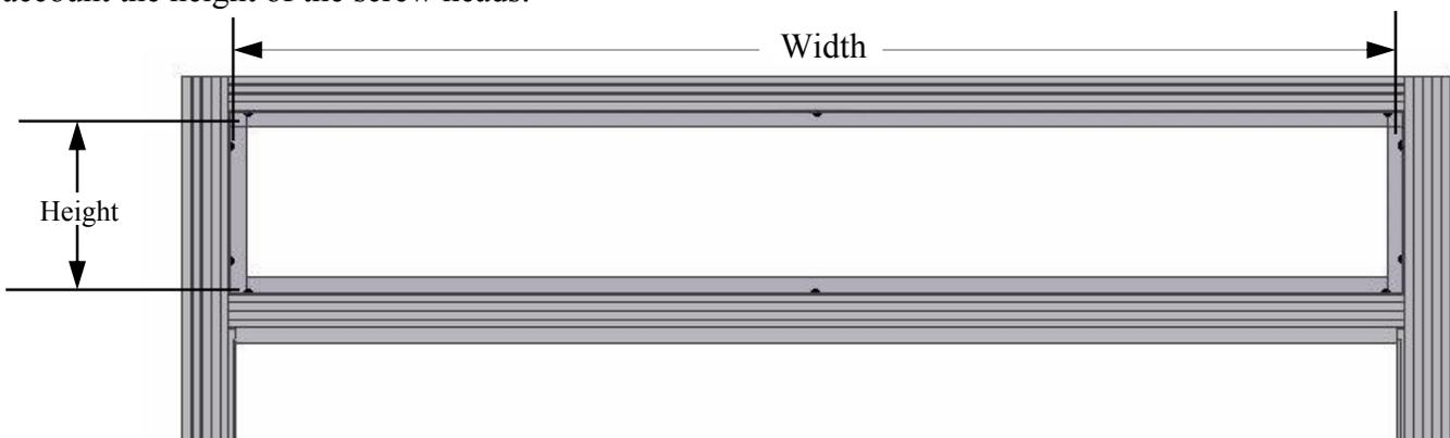
9) When you receive the **TEMPERED** Insulated glass from the glass supplier put Caulk on the face of the glass close to the edge and press the glass into place. Use the same procedure as in step 5 and enclose the glass with the 1" X 1" Angle using Caulk and #8 X 1/2" screws.
