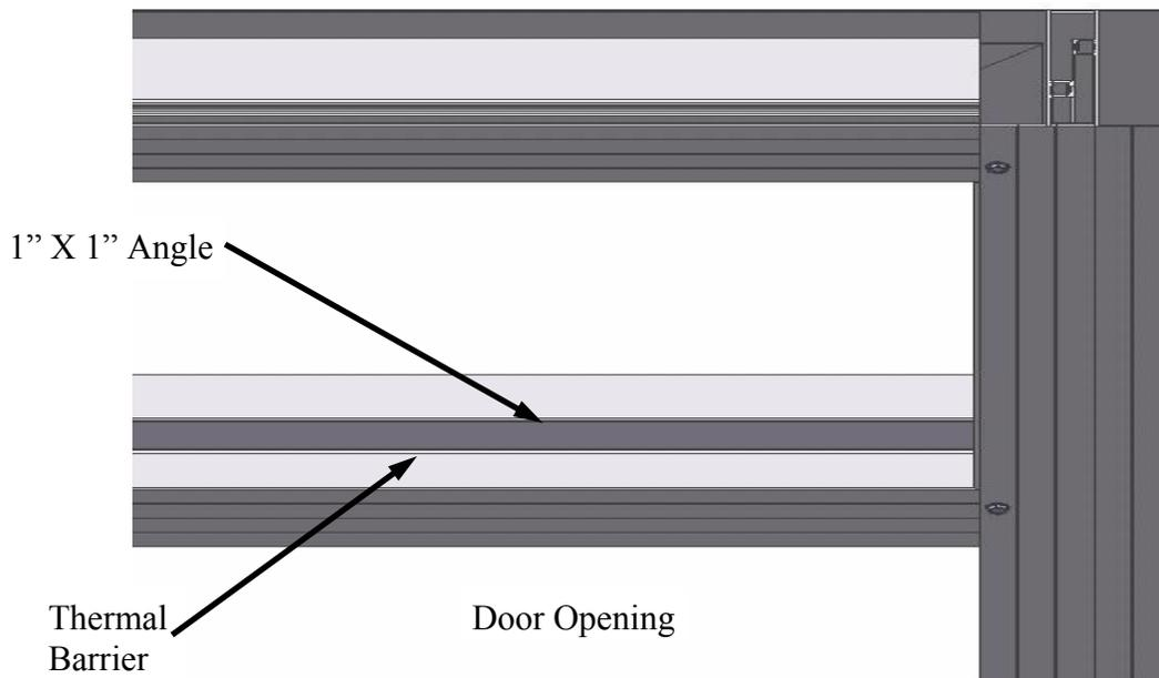
7 ) Using the 1” X 1” Angle cut your two side pieces. Caulk and position against the top and bottom Angles. Attach the Angle with #8 X 1/2” screws.
