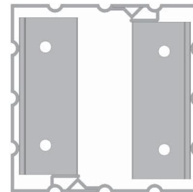
Locate positions on patio or deck for the two Column Angle Brackets. The Brackets must be positioned so solid sides (not joined sides) of the Column will be attached to Brackets.
