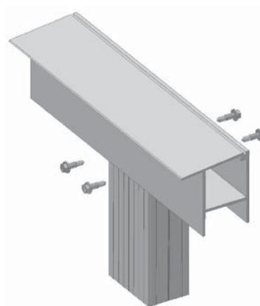
At each Column location install the Insert(s) (2" x 3" x 8") included with each Column. Push the Insert(s) to the stop in the Header and fasten with #12 x 3/4" Self Drilling Screws 1/2" up from the bottom of the Header and lined up with the second radius in from each edge on the Insert(s).
