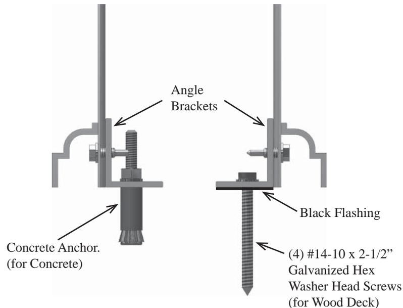
**Note: (2) of the #14-10 x 2-1/2" screws Require Full Embedment in wood Per Column.**
